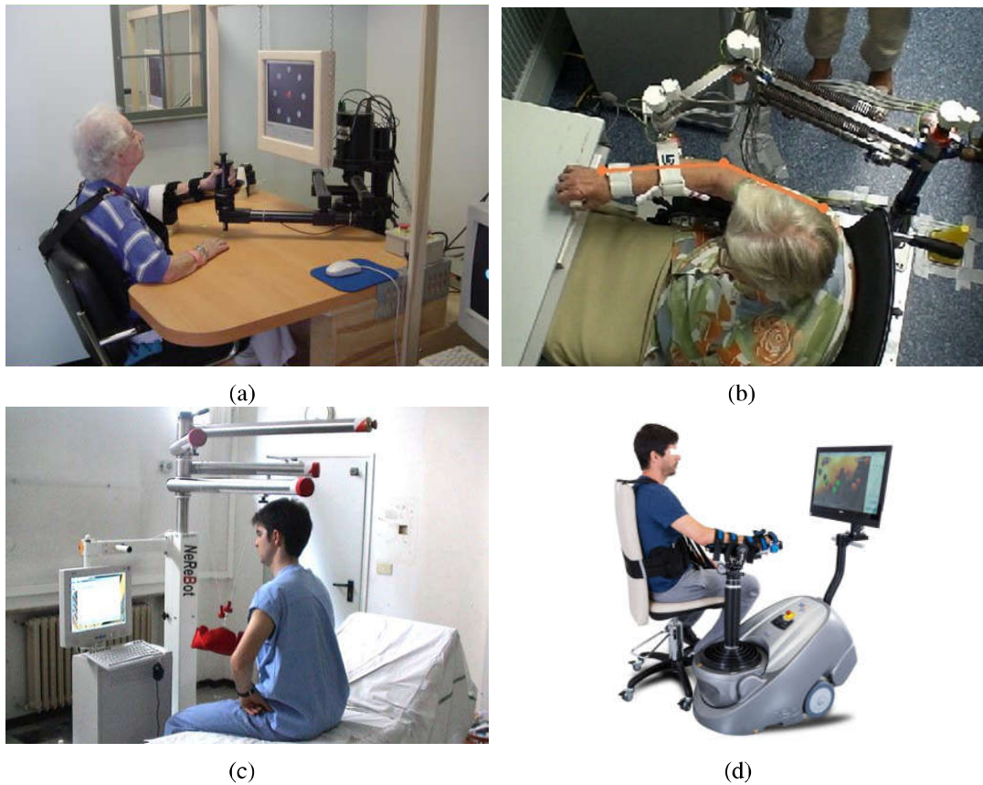
Figure 1.4: End-effector type robots for UE robotic rehabilitation, (a) Commercial version of the MIT-MANUS , the ACRE , (c) NeReBot , and (d) ReoGo [4–7].
